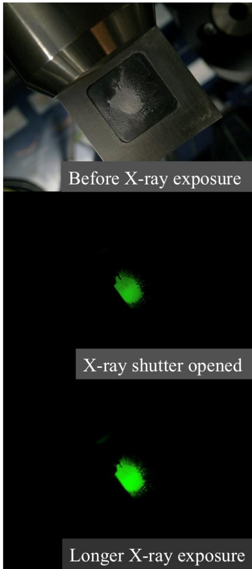
Figure 11.7. Preliminary scintillation tests showing how the \text{Cs}_3\text{TbSi}_4\text{O}_{10}\text{F}_2 scintillates under a Cu X-ray source.
