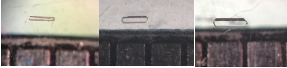
Figure A.1. Crystal images of the average size of \text{Na}_5\text{Er}(\text{OH})_6\text{WO}_4 (left), \text{Na}_5\text{Yb}(\text{OH})_6\text{WO}_4 (center), and \text{Na}_5\text{Tm}(\text{OH})_6\text{WO}_4 (right) crystals where the scale bar below the crystals denotes mm increments.
